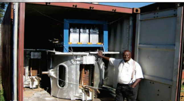
PROCURED ELECTRIC INDUCTION FURNACE TO BE INSTALLED AT CHAMBESHI PLANT
