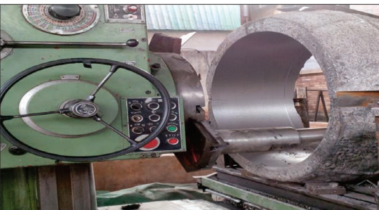
MACHINING OF BEARING HOUSING ON HORIZONTAL BORER
