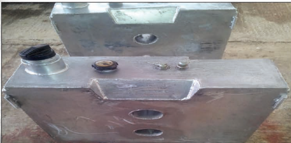
FABRICATED DIESEL TANKS FOR DANGOTE CEMENT PLANT
