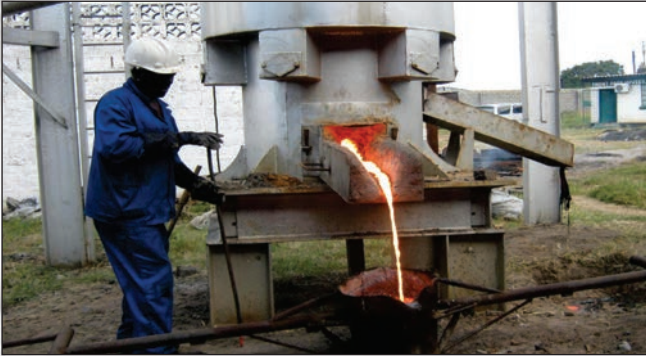
COUPLA FURNACE 2 TON CAPACITY
