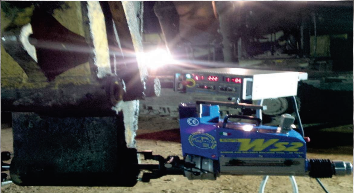
LINE BORING OF BOOM STICK AT CHINESE HYDRO PLANT
